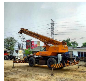
Rough Terrain Crane 25 Ton Tadano Crevo RK 250M-7
