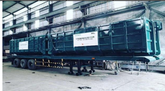
Semi-Trailer Arm Roll Box for Hazardous Material
