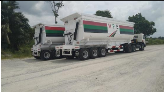
Semi-Trailer Side Dump Truck (SDT) Up to 120m 3
