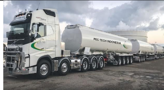
Superlink Triple Container for Caustic Soda (NaOH)
