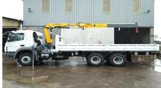
Truck Mounted Crane & 5-Way Flat Deck
