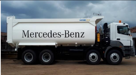
Rear Tipper Big 8x4 Dump Truck up to 45m 3
